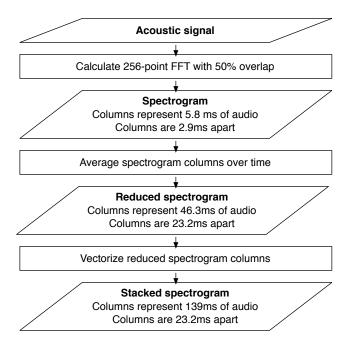
Fig. 2. Flowchart of the stacked spectrogram calculation.
