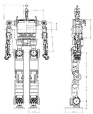
Figure 1: Hubo Schematic
